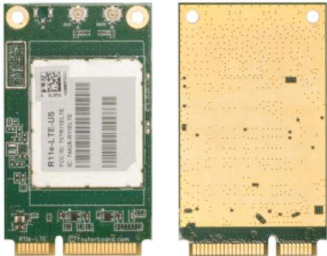
R11e-LTE-US is a Cat-4 modem. It can be integrated into any MikroTik product that has a miniPCI-e slot.
