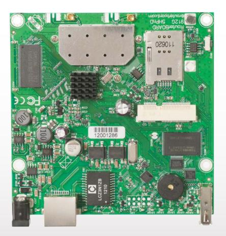
The RB912 is a small wireless router with an integrated high power wireless card and an additional miniPCle slot for 802.11 wireless, or 3G card. Both 2GHz and 5GHz models are available. The Gigabit port helps to utilize the full potential of 802.11n wireless speeds.
